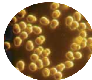
Figure 4b: Microscopic examination reveals anomalous particles: fused doublets of similarly sized particles.
